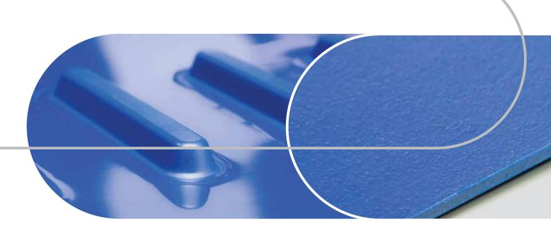
This new, monolithic lug drive belt is abrasion-resistant on both sides and easy to clean. It's made of thermoplastic polyurethane (TPU) with strong, aramid polymer cords for long-lasting stability. One side has a smooth adhesive surface and the other has an "orange peel" surface with a lower coefficient of friction than our standard lug drive product, CD.M40. This is the perfect belt for bakeries, dairies, fruit, meat, poultry or vegetable processing.
