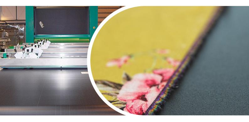
The new PB-2886 performance aramide printing blanket is specially designed for textile printing applications with regular and long printing tables. It provides high geometrical stability with improved lateral stiffness. It is also a suitable solution for very long flat bed printing machines as well as for magnetic system rotary machines with more than 15 colors.
