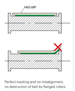
Some competitor belts, e.g. pure polyamide foils, are prone to fiber attraction and misalignment. This can lead to destruction of the belt edges by the flanged rollers, requiring early belt replacement in many cases.
