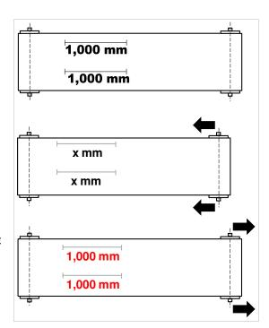
This method makes sure that the blanket is tensioned to the correct percentage related to its un-tensioned length.
