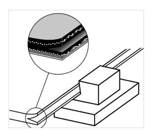
Slight deviations from straight running of the edge of a newly installed, untrimmed blanket are normal. This is why printing blankets are normally edge-trimmed after running in. This is especially important if automatic tracking control devices are used that have a sensor on the edge of the printing blanket.
