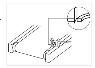
With the edge now perfectly trimmed, automatic control devices can now be switched on. Guiding blocks can be positioned at the blanket edges with a small clearance (on average 0.2 mm on both sides, a little more at the in-feed area). Check the clearance periodically. Re-track the printing blanket and restore it if the clearance becomes too large or too small.
