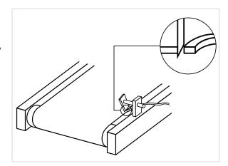
With the edge now perfectly trimmed, automatic control devices can now be switched on. Guiding blocks can be positioned at the blanket edges with a small clearance (on average 0.2 mm on both sides, a little more at the in-feed area). Check the clearance periodically. Re-track the printing blanket and restore it if the clearance becomes too large or too small.
