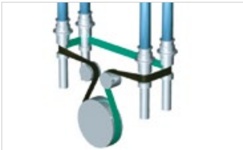
W-8/DS-8 four-spindle drive with two jockey pulleys
