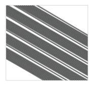
What's special about HabaSYNC® Flex timing belts is the variable arrangement of the cords inside the belt.
